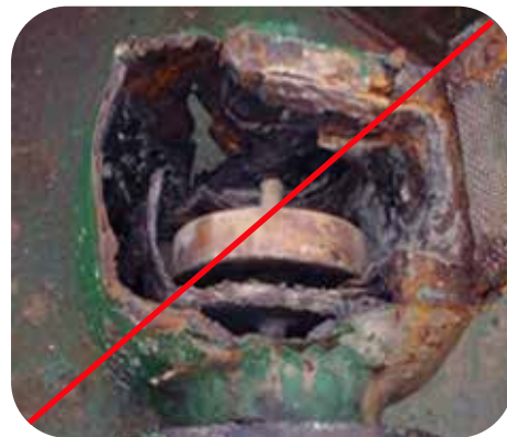
Watertight doors, air vents and windows not acceptable
