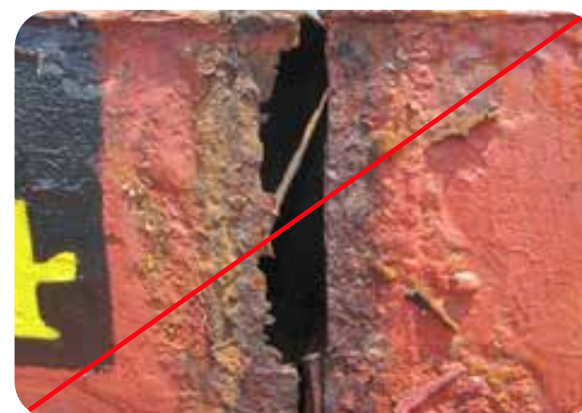
Hatch covers and weathertight closing appliances not acceptable – Gap, wasted hatch way, heavy corrosion
