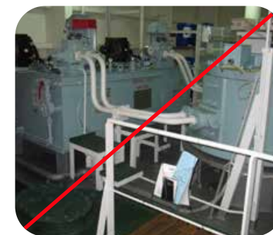
Steering Gear with Hyd. Oil Leak Not acceptable / Acceptable
